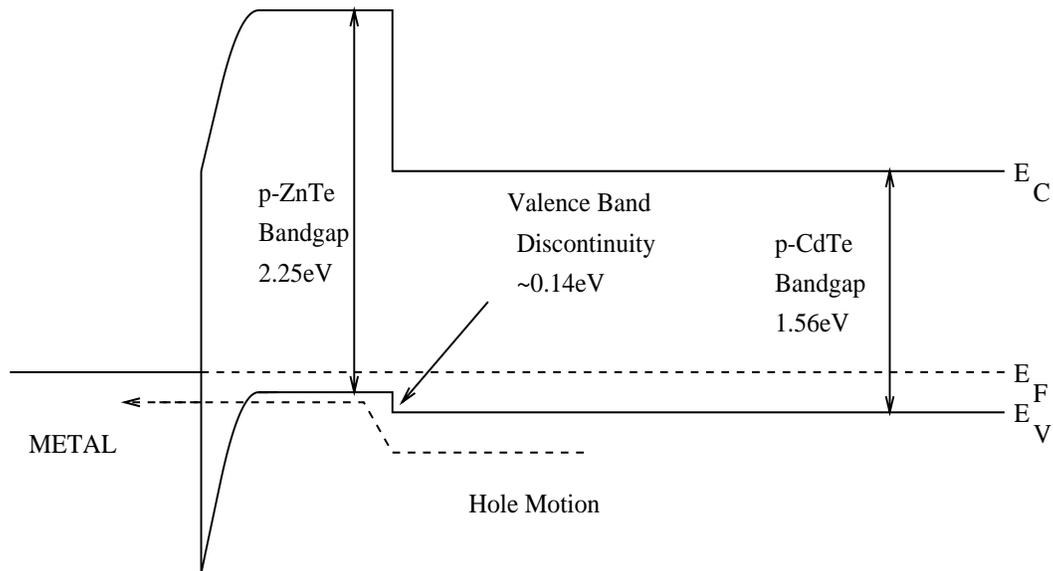
Figure 22 Band Diagram of CdTe/ZnTe Interlayer
