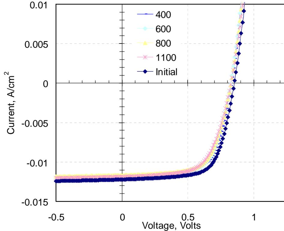
Figure 41 Light I-V Curve of the Same Device at Various Stress Times
