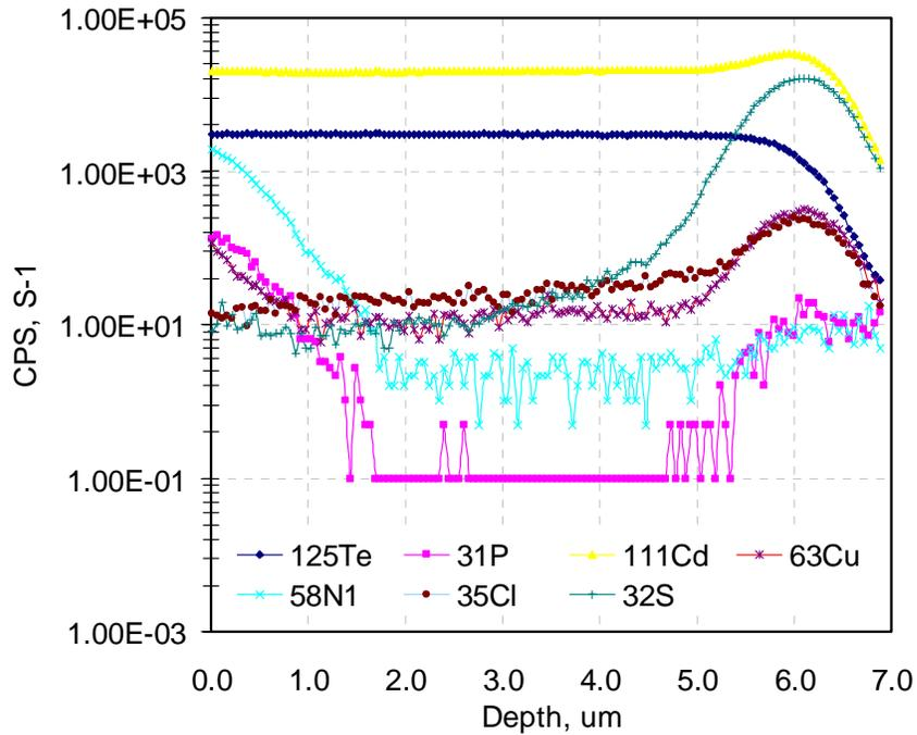
Figure 39 SIMS Depth Profile of a Cu Contacted Cell
