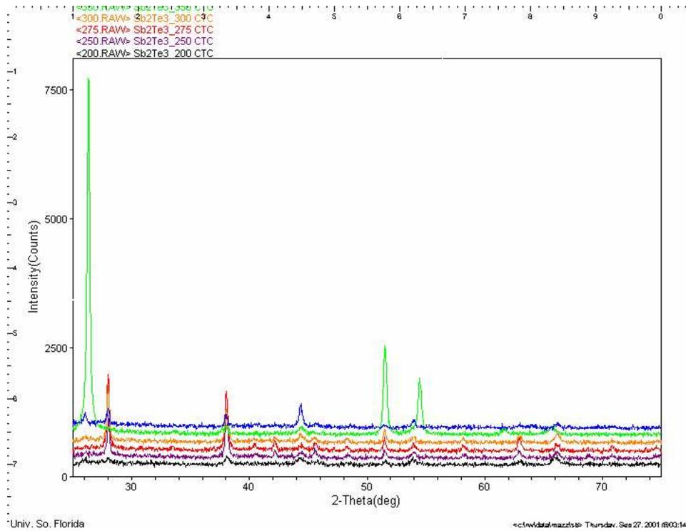
Figure 31 XRD Patterns of  $\text{Sb}_2\text{Te}_3$  Films at Various Temperatures
