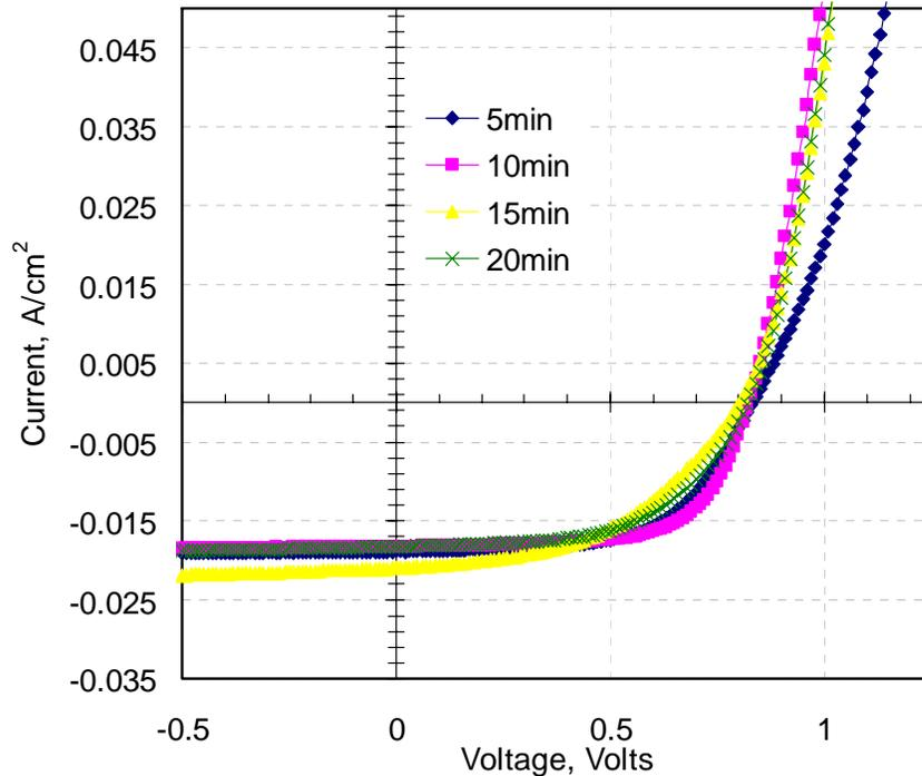
Figure 46 Effect of Plasma Power of 75 W on the J-V Characteristics
