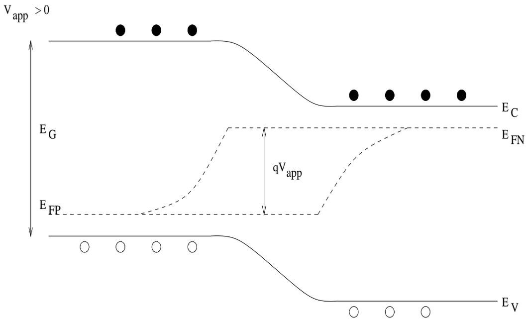
Figure 10 P-N Junction Under Forward Bias
