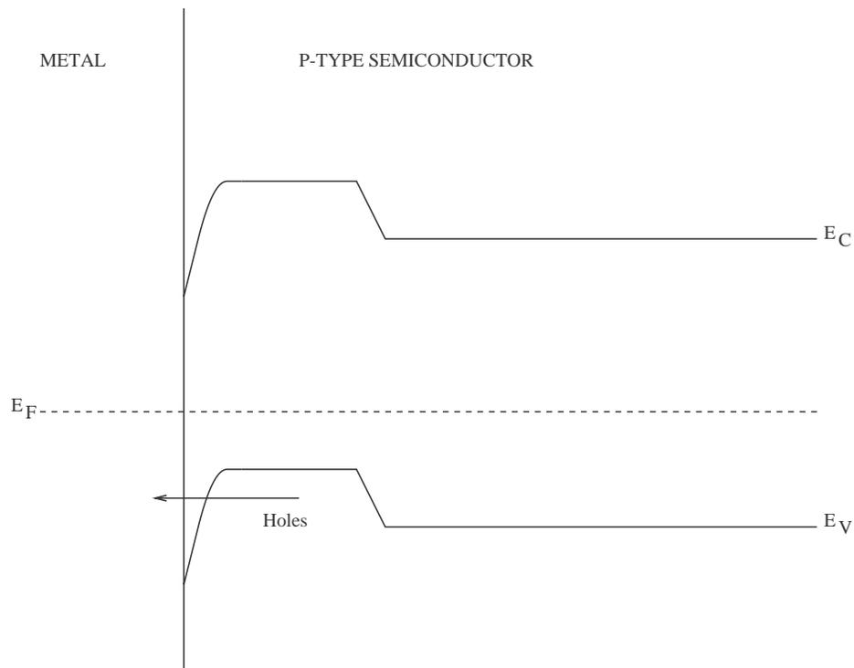
Figure 7 Energy Band Diagram of Metal-Semiconductor Tunneling Contact
