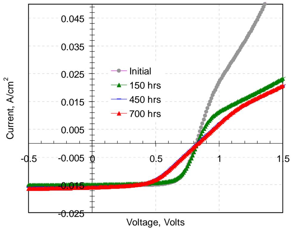
Figure 29 J-V curves of Same Device with Stress Time (70°C)
