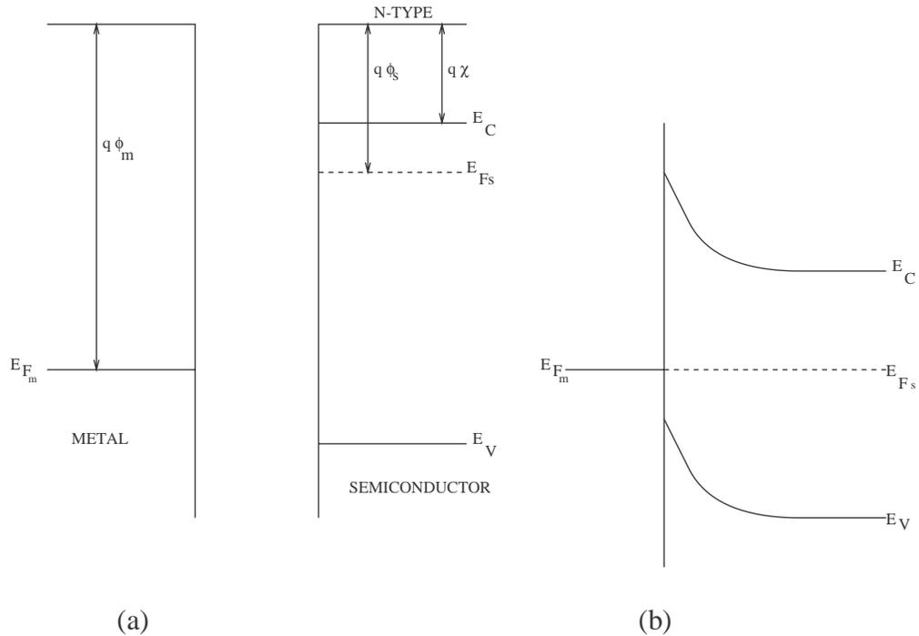
Figure 1 (a) Band Diagrams of Metal and Semiconductor before Junction Formation, (b) After the Junction Formation
