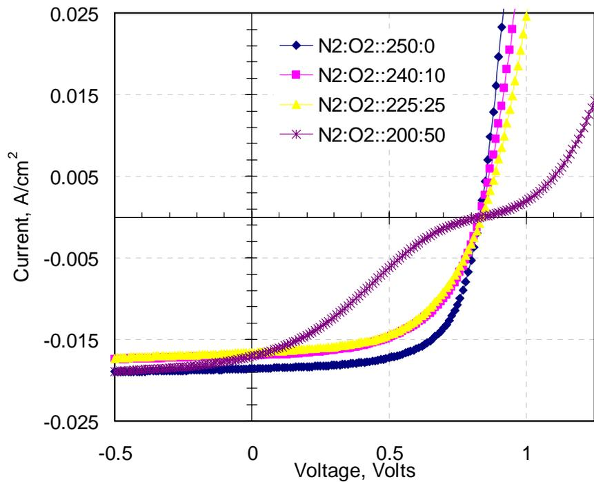
Figure 49 Effect of Increased O<sub>2</sub> Partial Pressure on J-V Characteristics
