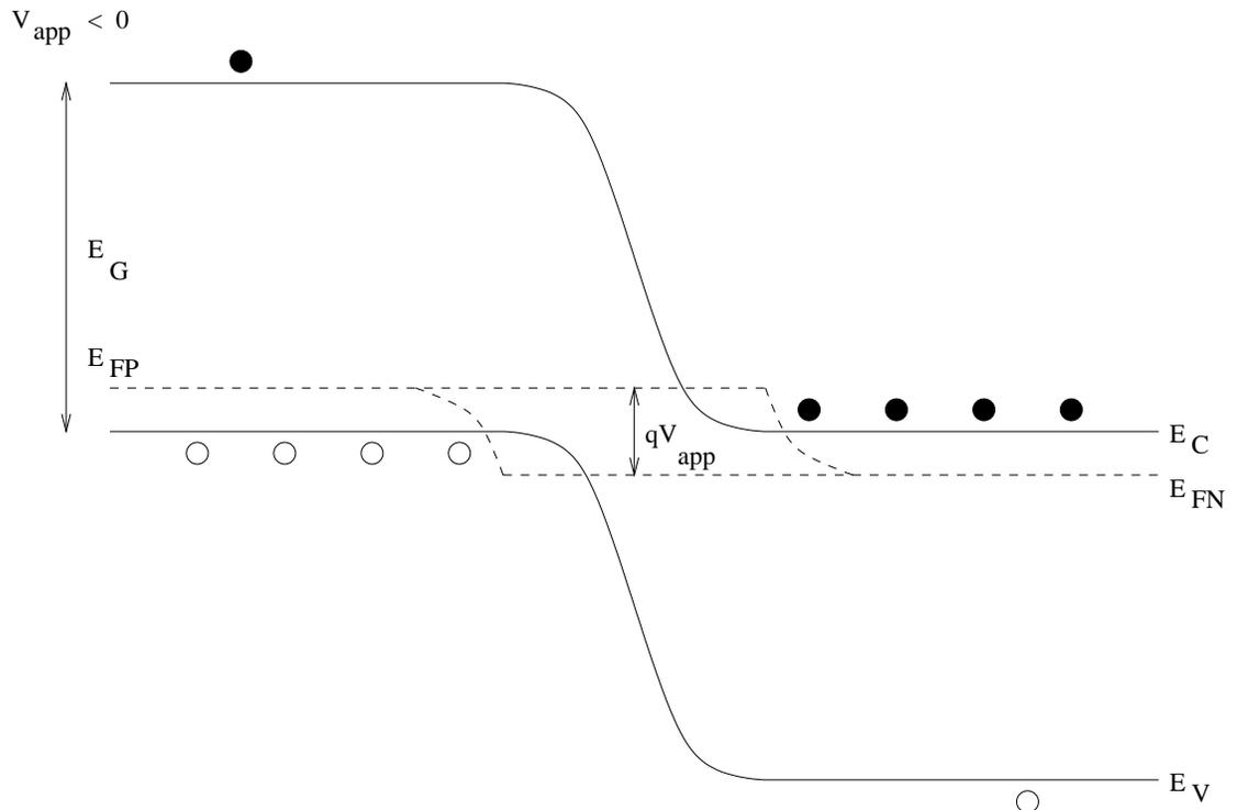
Figure 11 P-N Junction Under Reverse Bias
