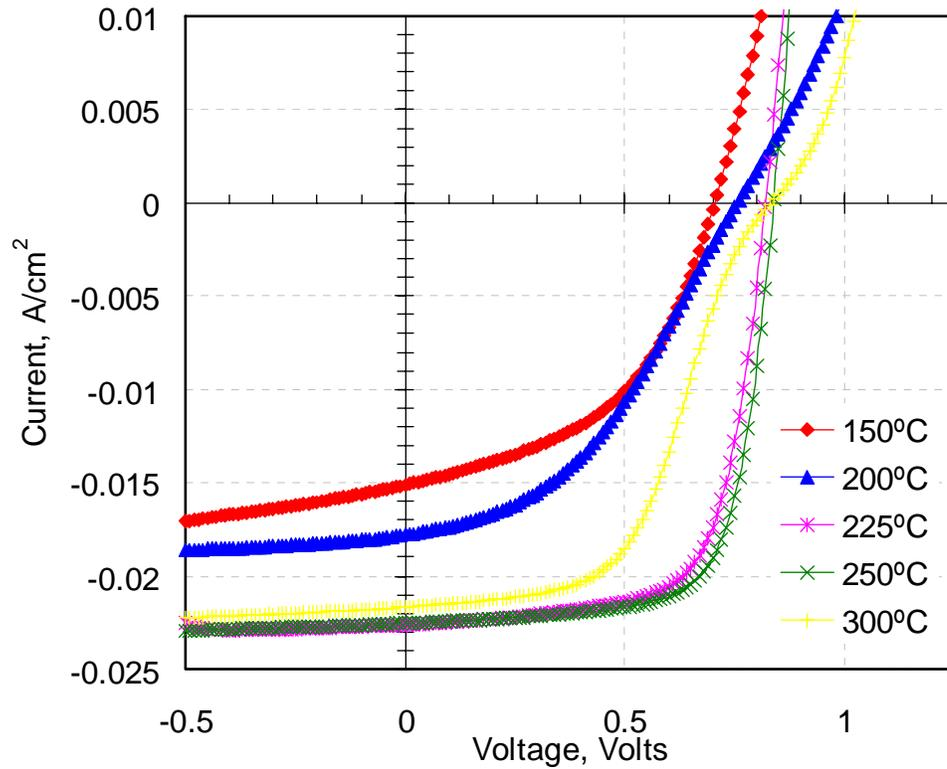
Figure 36 Effect of Contact Annealing Temperature on J-V Curve
