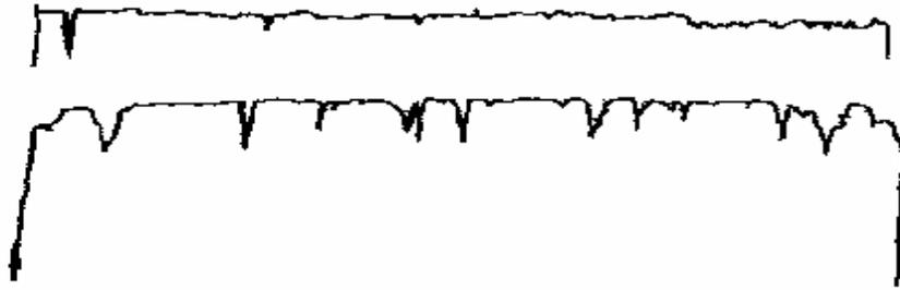
Figure 24 OBIC Scans of CdTe Cells with  $\text{Cu}_x\text{Te}/\text{Mo}$  (top) and Graphite (bottom) Contacts
