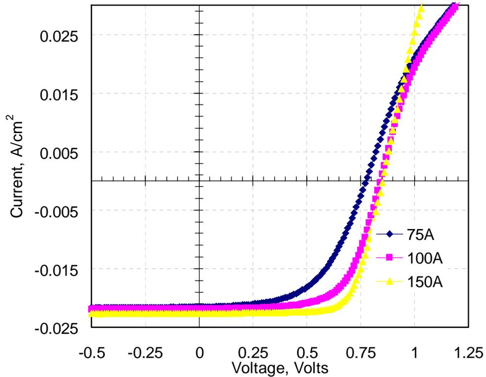
Figure 27 Effect of  $\text{Cu}_2\text{Te}$  Thickness on J-V Characteristics
