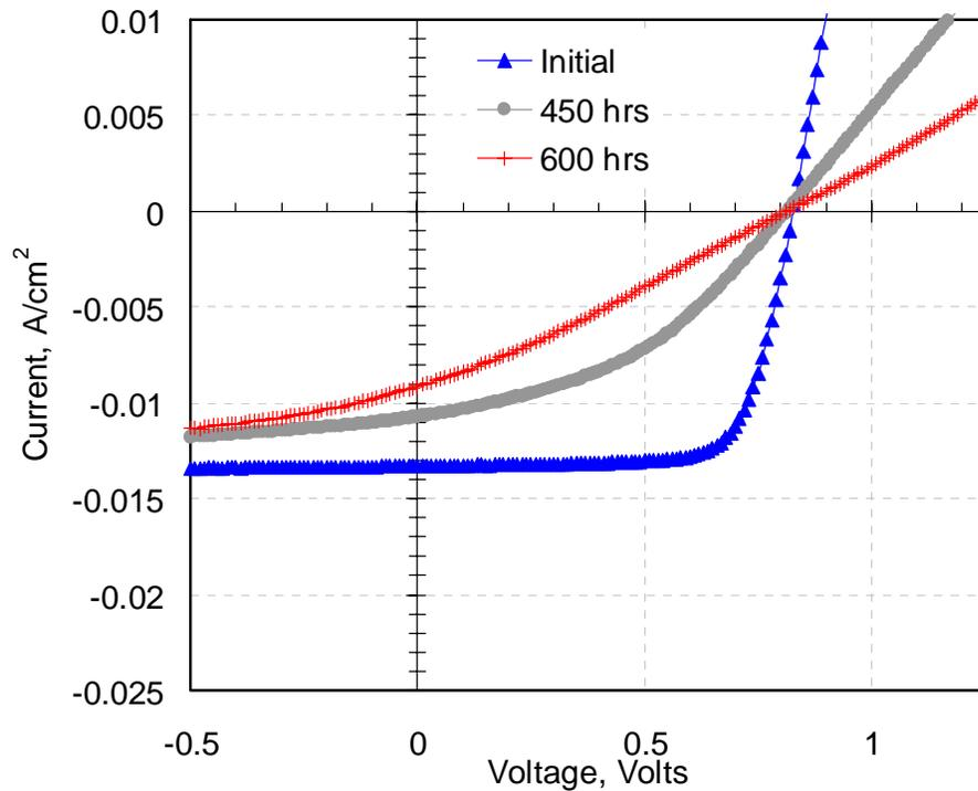
Figure 30 J-V Curves of Same Device with Stress Time (100°C)
