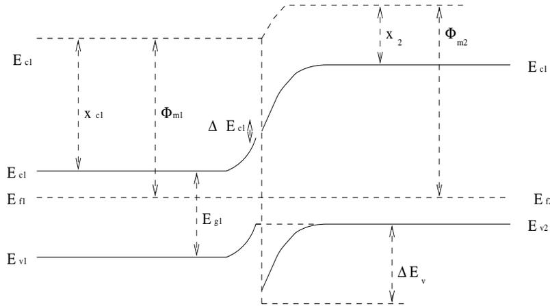
Figure 16 P-N Heterojunction
