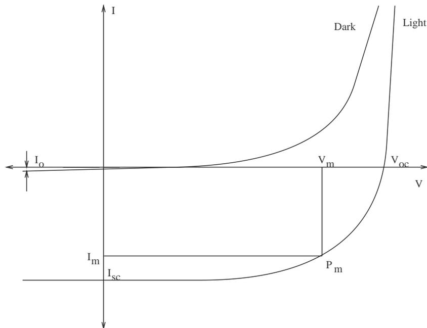
Figure 12 I-V Curve of the Solar Cell in Dark and under Illumination
