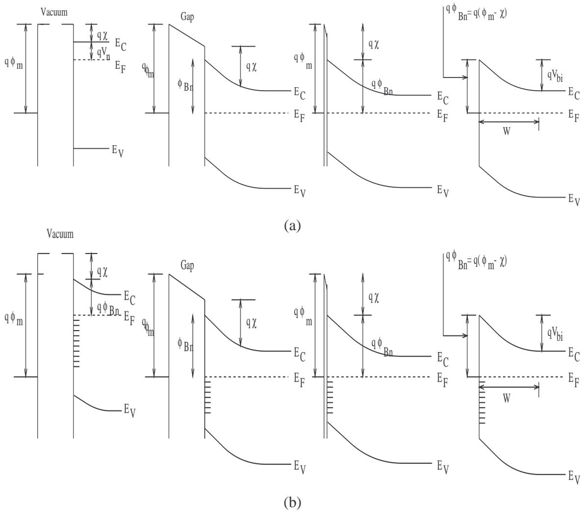
Figure 3 (a) Band Diagram of Metal - Semiconductor in the Ideal Case, (b) With Surface States
