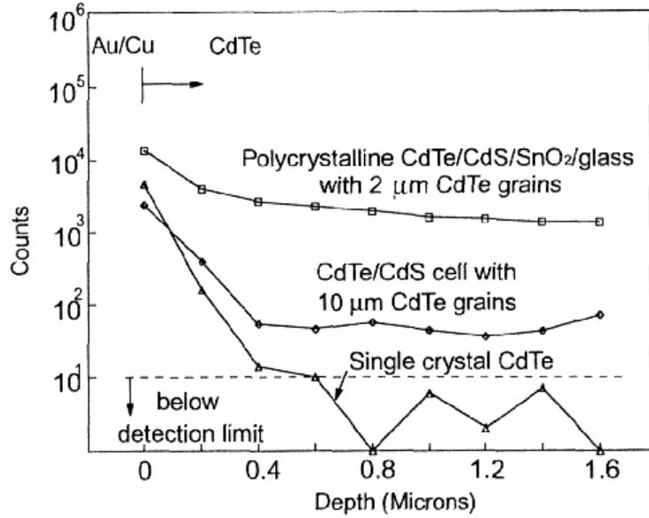
Figure 20 Cu SIMS Profile in the CdTe Layers with Different Degrees of Crystallinity
