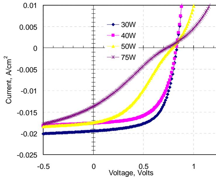
Figure 48 Effect of Plasma Power on J-V Curve using Ar as the Etching Ambient
