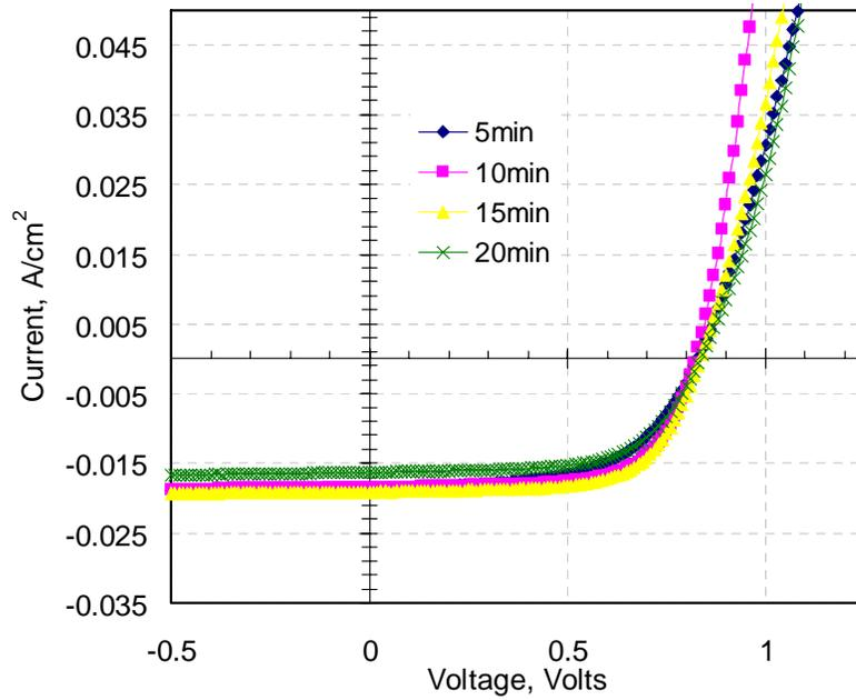
Figure 45 Effect of Plasma Etch Time on J-V Characteristics(50W)
