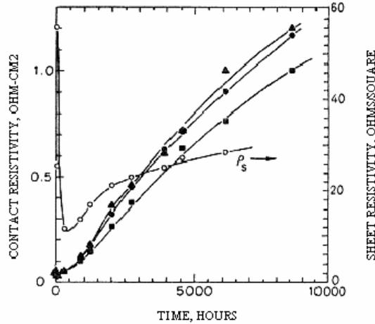
Figure 21 Contact and Sheet Resistivity for Li Diffused Contact on CdTe
