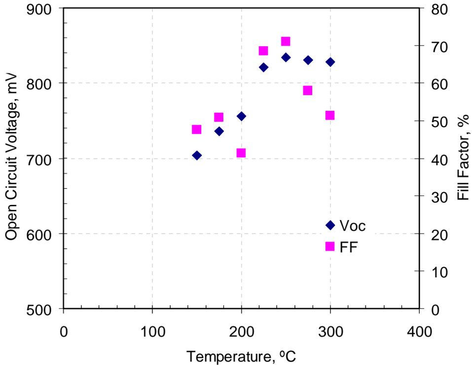
Figure 35  $V_{oc}$  & FF as a Function of Anneal Temperature
