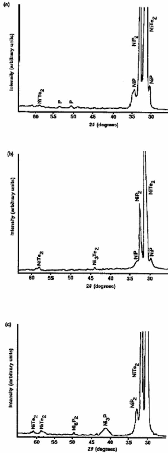
Figure 4. X-ray profiles of a Ni-P/CdTe contact (a) just after deposition, (b) after annealing at 250 °C for 90 min and (c) after annealing at 350 °C for 50 min.
