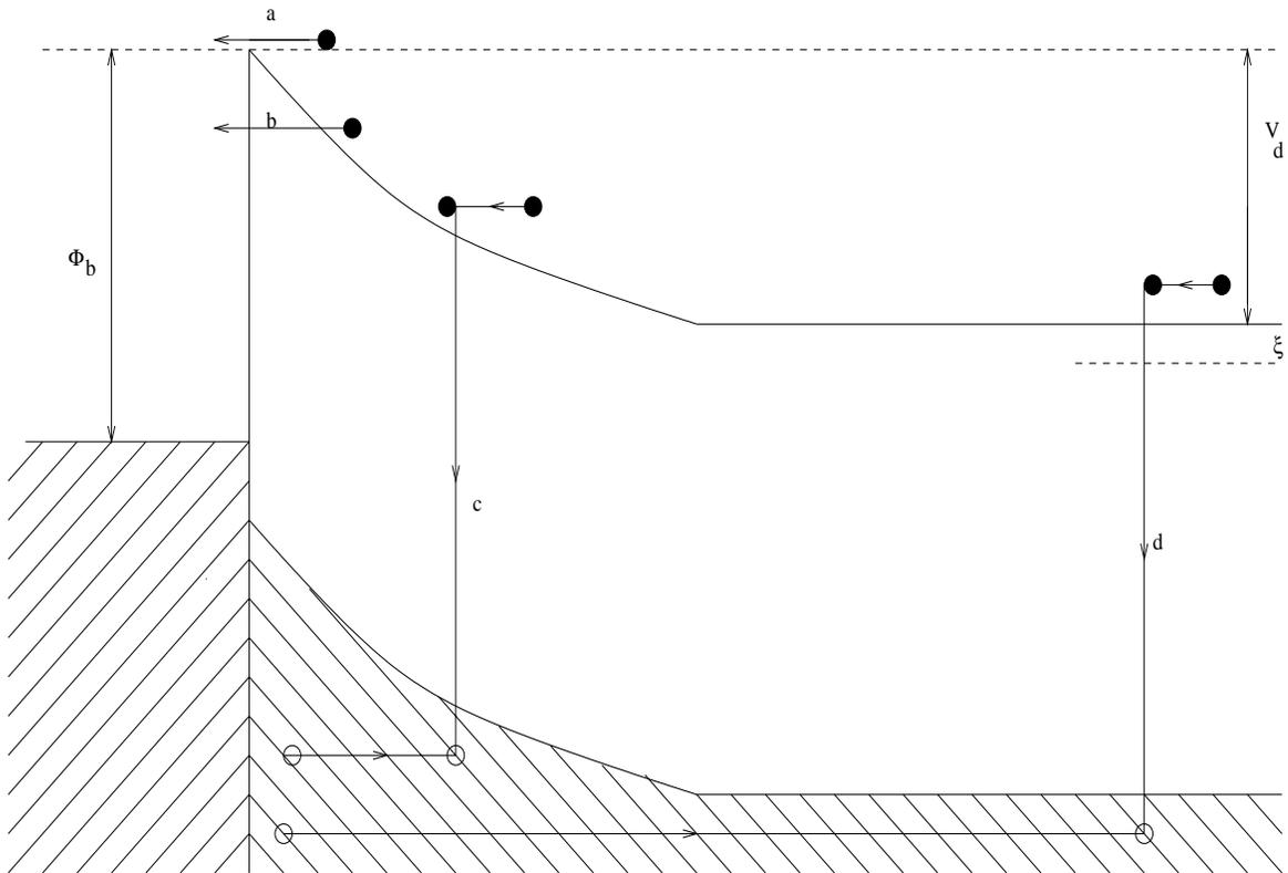
Figure 5 Current Transport Mechanism (Forward Bias) in Metal–Semiconductor Contacts
