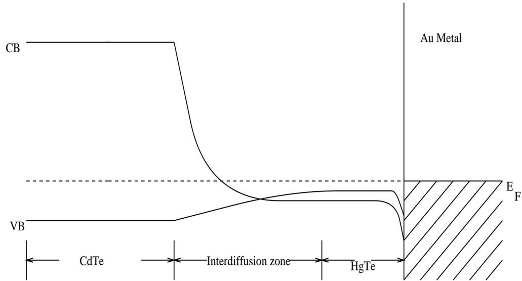
Figure 23 Equilibrium Energy Band Diagram of CdTe/HgTe/Au Interface
