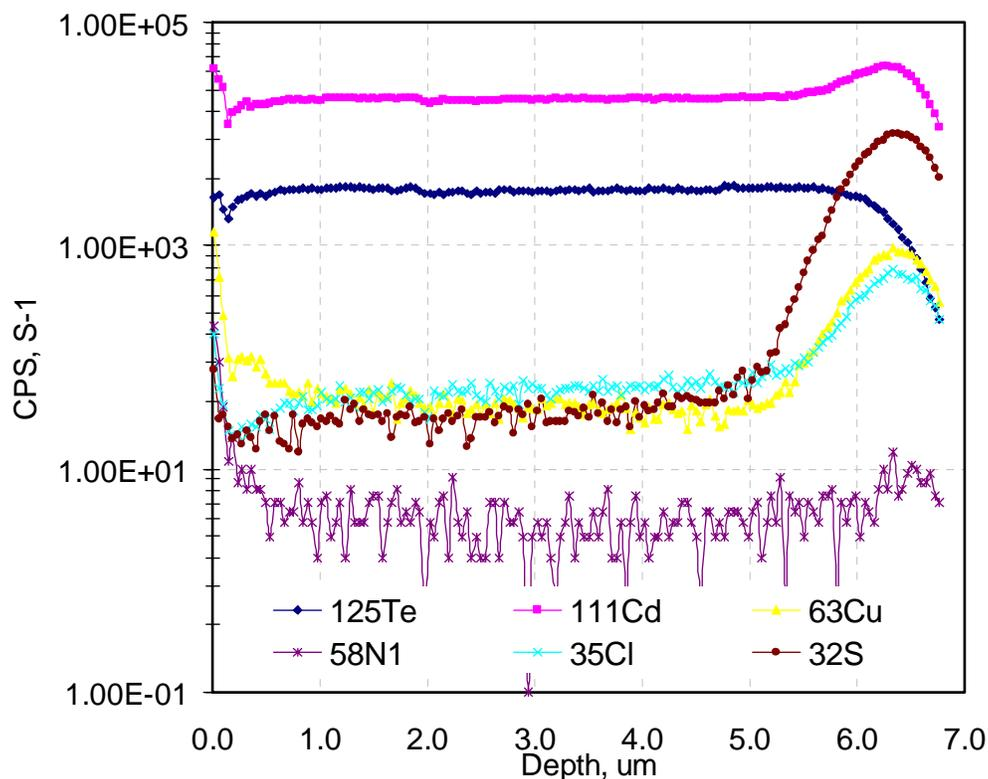
Figure 38 SIMS Depth Profile of a Ni<sub>2</sub>P Contacted Cell
