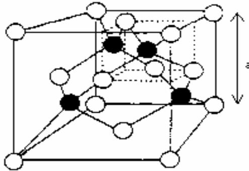
Figure 18 CdTe-Zinc Blende Structure
