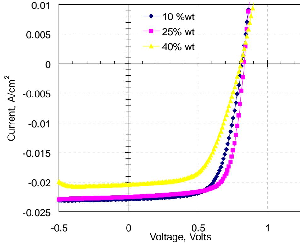
Figure 34 Effect of Ni<sub>2</sub>P Concentration on the J-V Curve
