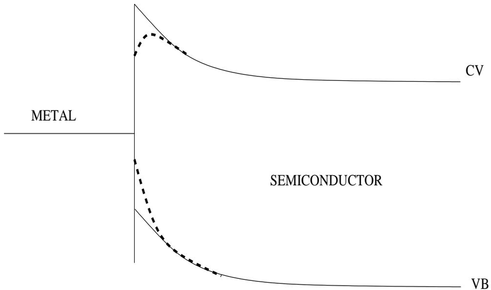
Figure 6 Effect of the Image Force on Barrier Height
