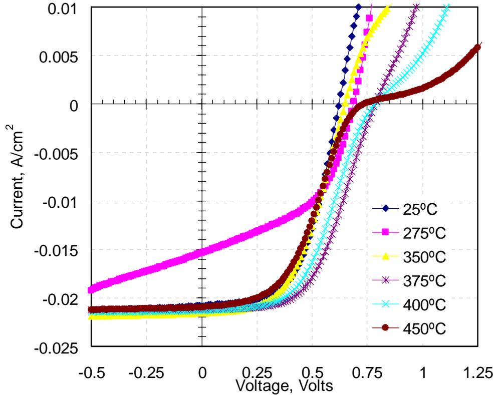
Figure 32 Effect of  $\text{Sb}_2\text{Te}_3$  Deposition Temperature on J-V Curve
