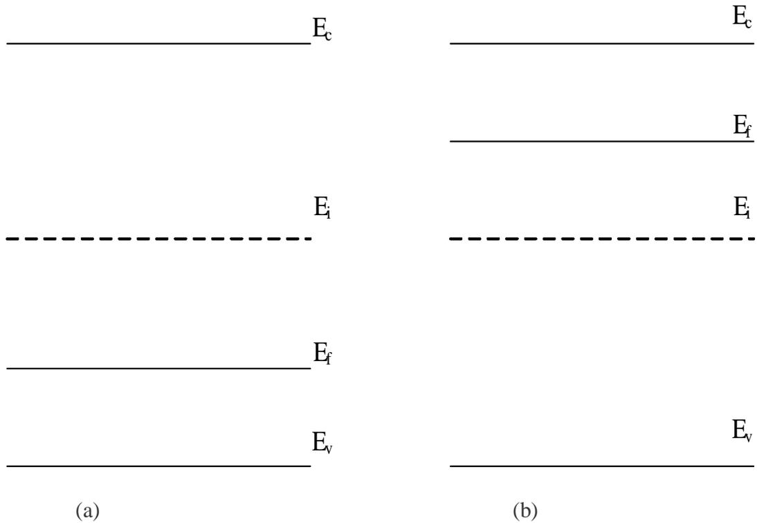
Figure 8 Band Diagrams of (a) P-type, (b) N-type Semiconductors
