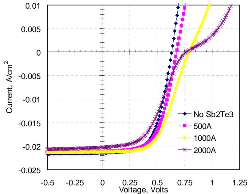
Figure 33 Effect of  $Sb_2Te_3$  Thickness on J-V Characteristics
