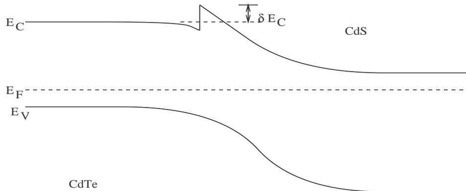
Figure 19 Spike at the CdS/CdTe Heterojunction
