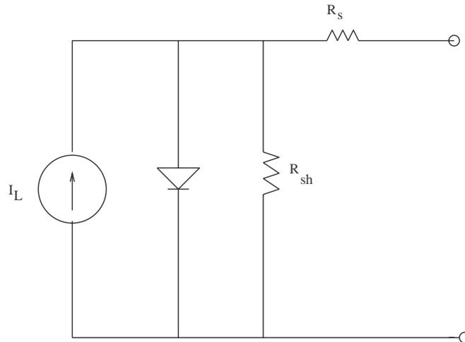
Figure 14 Equivalent Circuit of a Solar Cell
