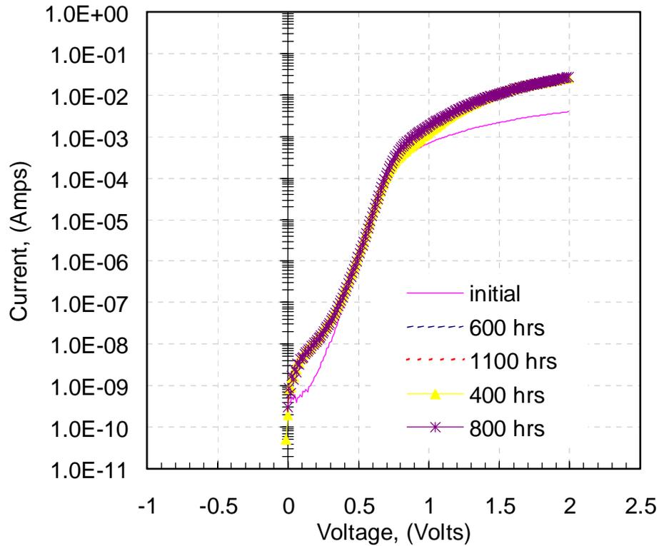
Figure 40 Dark J-V curve of Stressed Devices at Various Stress Times
