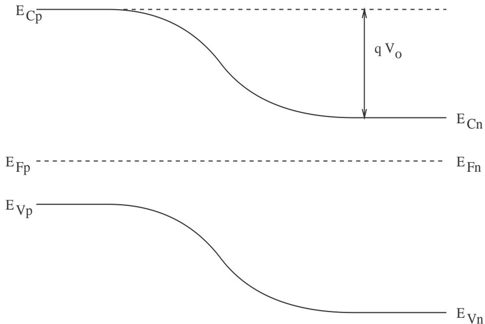
Figure 9 Band-Bending at the Junction
