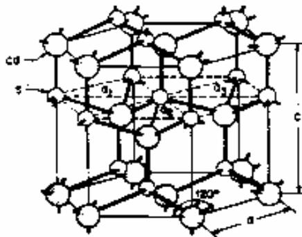
Figure 17 Hexagonal Structure of CdS
