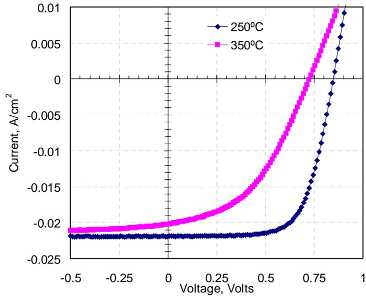
Figure 28 Effect of Cu<sub>2</sub>Te Deposition Temperature on J-V Characteristics
