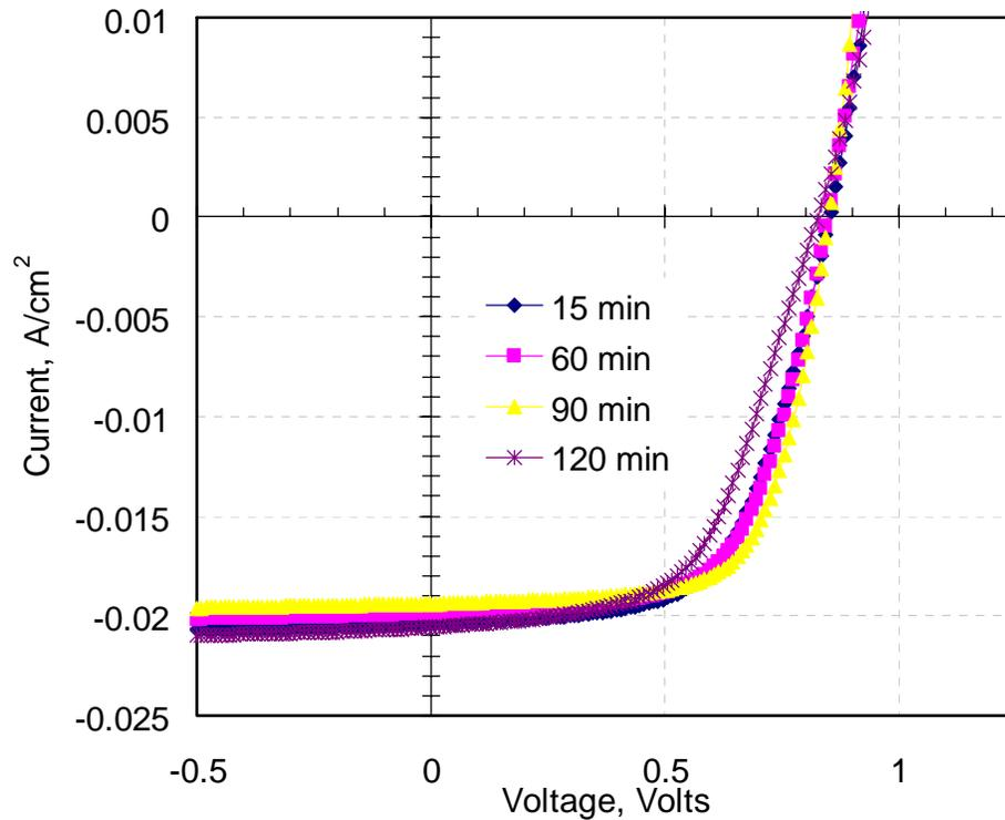
Figure 37 Effect of Annealing Time on Contact Properties
