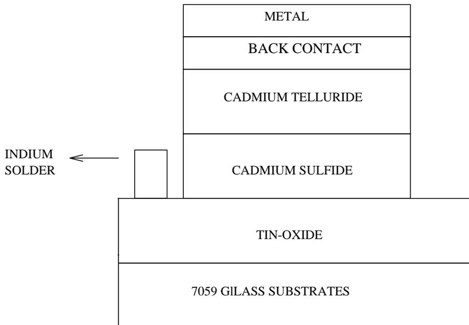
Figure 26 Schematic of CdS/CdTe Solar Cell (Superstrate Structure)
