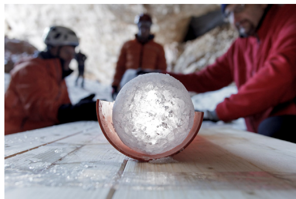
Figure 1. One sector of the ice core just extracted from the Vasto ice cave. Photo courtesy Fabrizio Giraldi.
