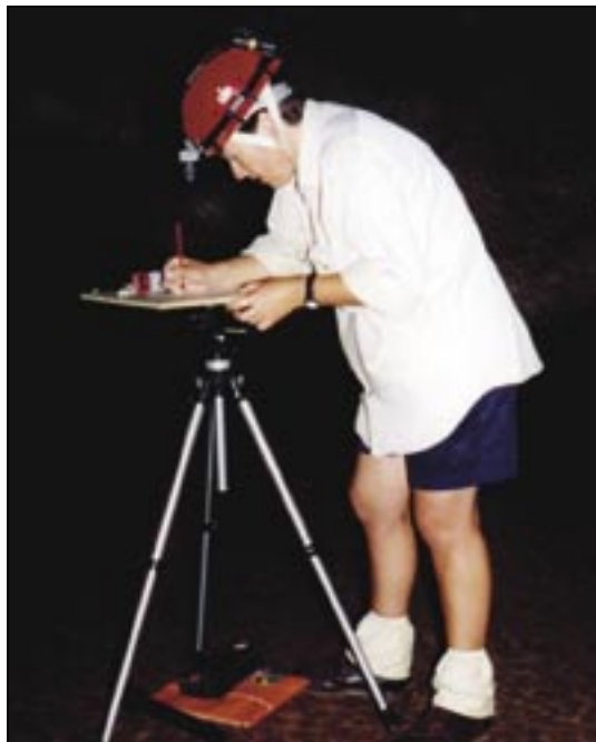
Fig. 18: Claire Cooney using a plane table and laser rangefinder at Wellington Caves.
