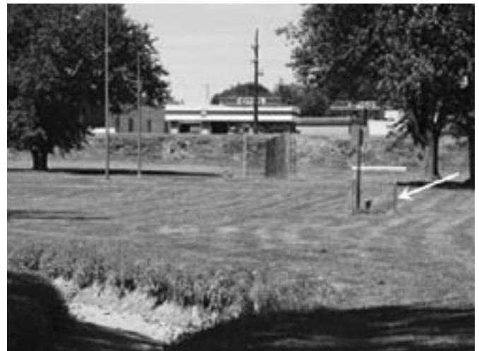
Fig. 1. Unnamed normally dry stream channel in a karstic terrane during extended periods of little or no precipitation. Note production test well surrounded by safety fencing (arrow) and gasoline service station in background (service station is upgradient of creek).
