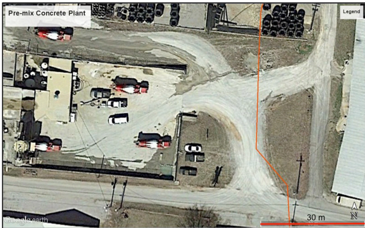
Figure 5. Google Earth Image March 2014. Premix concrete plant in Horse Cave. Runoff from the site follows the purple line that terminates at an open drainage well. The orange line represented the underlying cave passage, suggesting ~25 m mis-registration.
